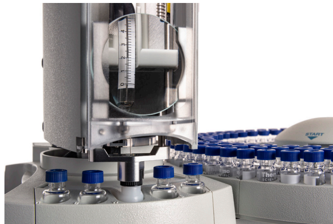
AI/AS 1610 syringe compartment with magnifying lens
